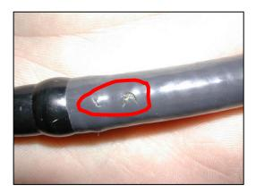
Tooth Drag Marks on Insertion Tube Sleeve
